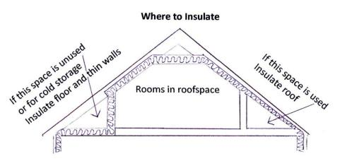
If these areas are not insulated, heat from the rooms below will escape through the ceiling and then straight through the roof. Heat will also escape from any adjoining rooms, through the thin timber partition walls. How you insulate these areas depends on what these areas are used for. If there is no access it could be worth having one or more hatches cut to gain access to these sections.
